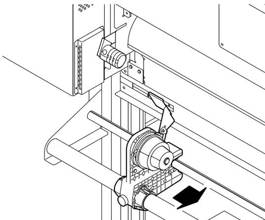
(2) Check the clamp lever is lowered.
